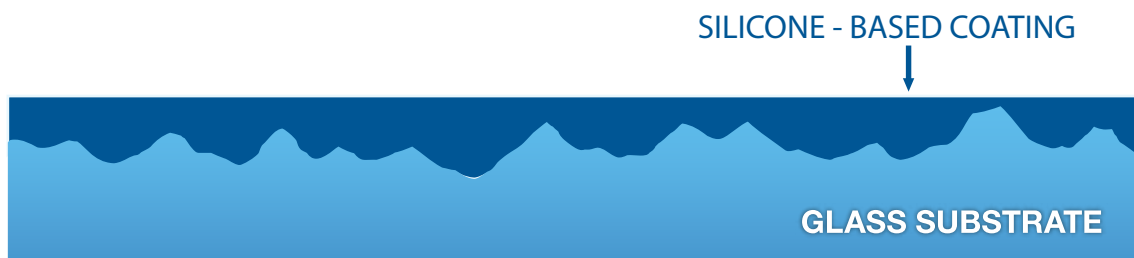
Fig 1. Competitive products that fill in the hills and valleys of the glass
